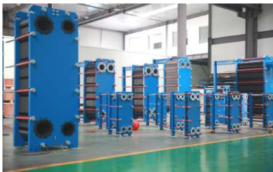
Plate Heat Exchanger
