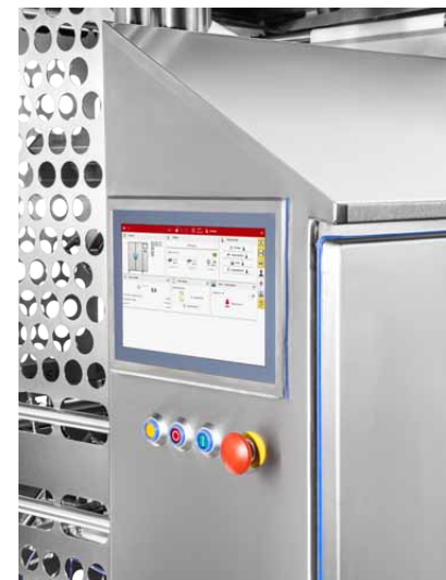
Full color touch screen with Industrial PC
