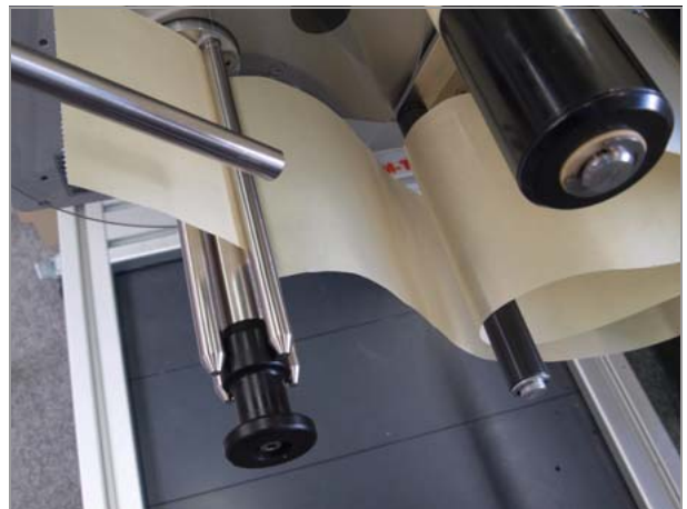
[46] Inserting the end of the backing paper into the rewinder.
