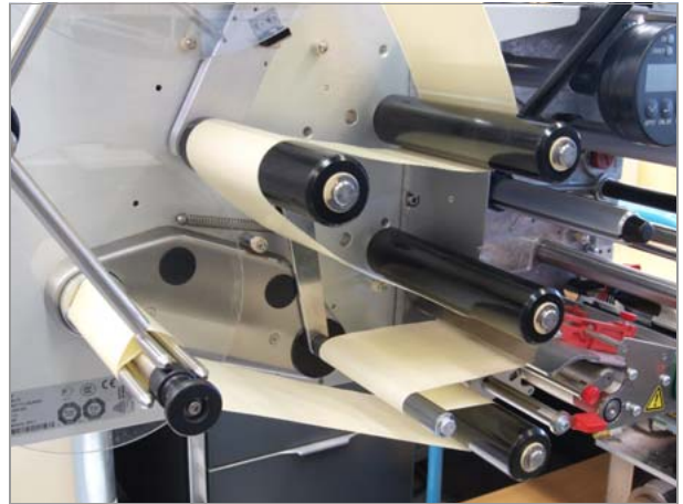
[45] Threading the backing paper on the rewinder.
