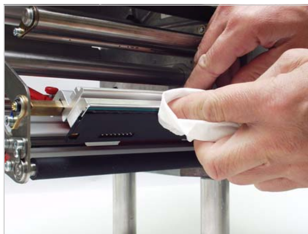
[65] Clean the printhead with alcohol.
