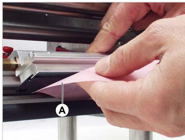
[64] Clean the printhead with the cleaning strip.
