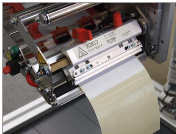
[41] Peel the labels off on a length of 50 cm.
