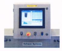
**Designed to Food Industry Standards**Fully enclosed and interlocked cabinet
