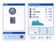
**15" Touch Screen Control Panel**Simple operation with complete diagnostics display and histogram
