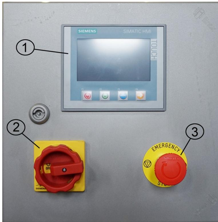
The control board in AISI 304 stainless steel encloses the electrical system, pneumatic system is at the rear of the machine:
