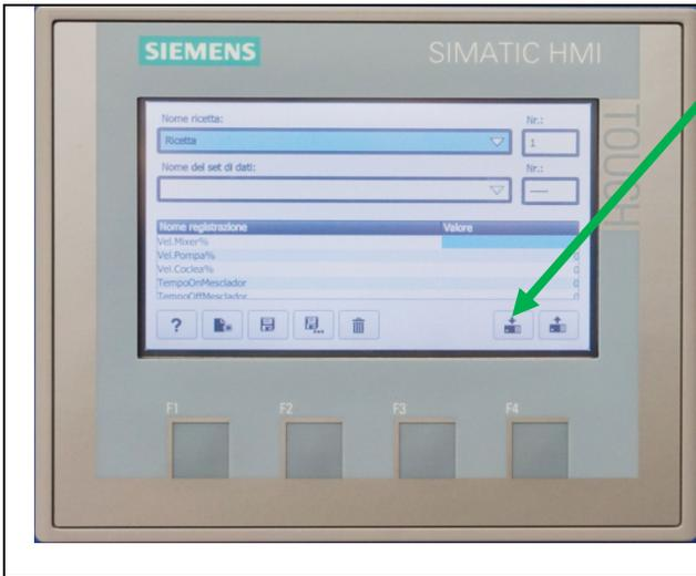
Pressing the “up arrow” command we go to pull out a recipe to PLC.
