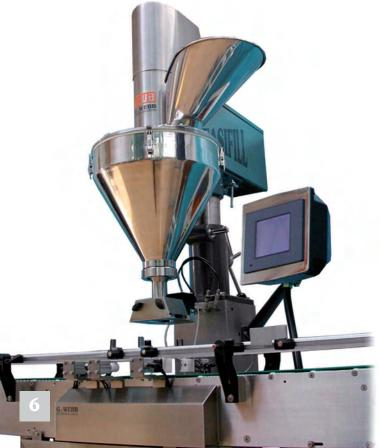
The EF-III 'EasiFill' range of auger filling machines brings to the user all the advantages of the latest direct drive filling technology providing servo drive flexibility for applications where outright servo drive performance is not required. The lack of clutches, brakes, belts and chains eliminates expendable items, and thus reduces maintenance to an absolute minimum. This can dramatically increase the long term reliability, especially with installations running continuous shifts.
