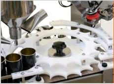
The 'RotoPlant' range, is designed for ultimate speed in container handling and filling. It is particularly aimed at powder & particulate packaging industry sectors, but is also extremely capable of handling larger particulates such as tablets, potato snacks & confectionery and is an attractive solution for pharmaceutical, chemical, and food ingredient companies using glass or composite containers, requiring clean & compact filling.
