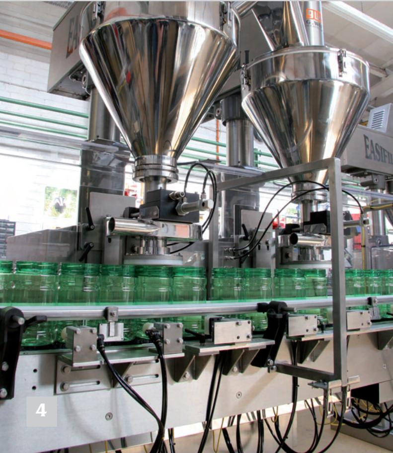
The 'RotoPlant' range, is designed for ultimate speed in container handling and filling. It is particularly aimed at powder & particulate packaging industry sectors, but is also extremely capable of handling larger particulates such as tablets, potato snacks & confectionery and is an attractive solution for pharmaceutical, chemical, and food ingredient companies using glass or composite containers, requiring clean & compact filling.
