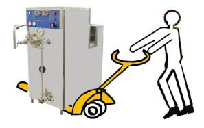
Move the machine using a manual pallet trolley. Insert the trolley forks either under the side or the front of the machine.
